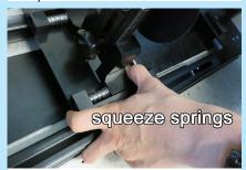
Your material must be completely locked in with all the levers and knobs tightened. A good way to ensure a tight fit is to first squeeze the spring on the left side.
