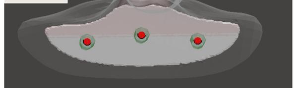
Drainage holes are needed for hollow Form 1+ models. Choose your number of holes per hollow, and then press “Generate holes”. Place the red dots by dragging them and press “Accept” to hollow.
