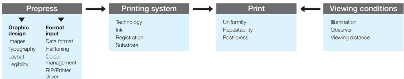
**Figure 1:** Factors determining print quality in digital printing processes
