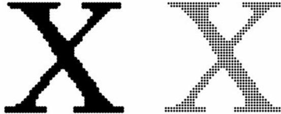
**Figure 10:** The effect of dot size on colour density
