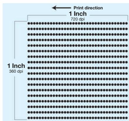
Figure 3: Xaar 1002 printhead with encoder resolution increased to give 360x720 dpi
