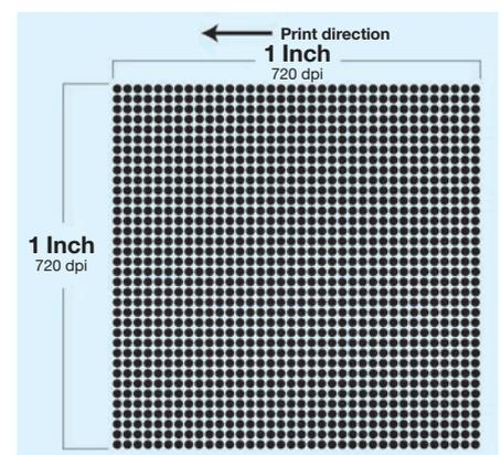
Figure 4: Xaar 1002 printheads interleaved to give 720x720 dpi
